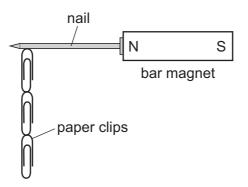
The bar magnet is then removed and the number of paper clips remaining attached to the nail is recorded. Each nail is tested individually.
